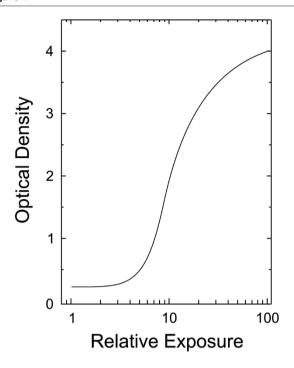
Characteristic curve of a screen-film mammography image receptor. There is an approximately linear relationship between optical density of the processed film and the logarithm of relative X-ray exposure, but only over a limited region of exposure.
