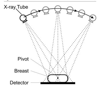
Schematic representation of image acquisition in breast tomosynthesis.
