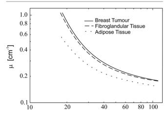
Linear X-ray attenuation coefficients of fat and fibroglandular tissue in the breast plotted versus X-ray energy. Values for samples of breast tumors are also shown. 'Reproduced from [51] with permission from IOP Publishing Ltd.
